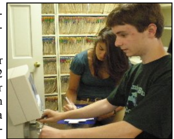
Chris Santucci and Taylor Skala measure eyeglasses with an automatic lensometer.
